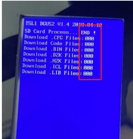
Figure Display status of failed firmware update on the display
